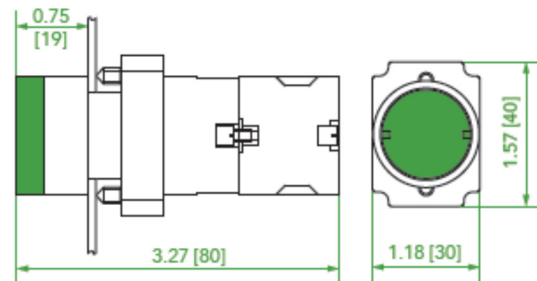
Ex9PBW3 Momentary Flush with Guard Unit: in [mm]
