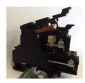
Double-level modular terminal block with suppressor diode as surge protection between both levels, hinge disconnect in the upper level, nominal voltage: 24VDC, for mounting on DIN 35 or DIN 35 mm rail, closed housing, terminal width: 8 mm, terminal height: 51.5 mm
