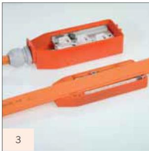
Position the fl at cable in the right position. The lug in the base acts as a reference point. It has to match the lug of the fl at cable. In case of incorrect mounting the box cannot be fitted with normal force. The cable must be cleaned, gel and oil must be removed.
