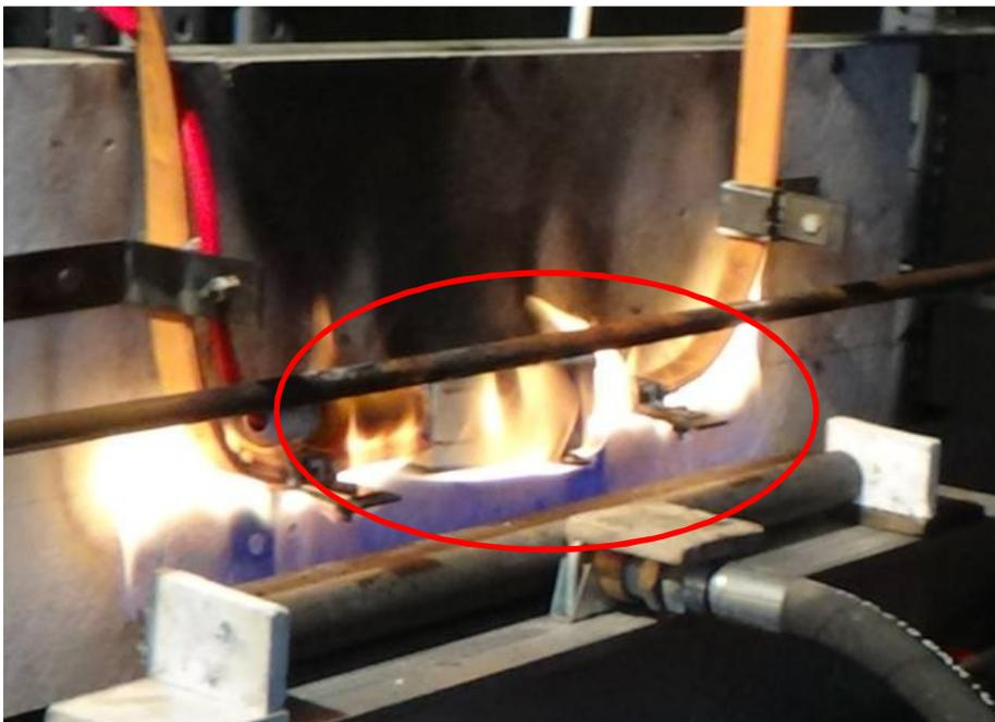
Junction box and the fuse module in the fire test BS8434-2
