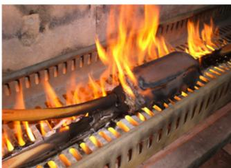
Testing the function integrity requires measuring the duration which current continues feeding life safety equipment such as emergency lighting, smoke extraction systems, alarms and exit signs.
