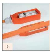
Position the fl at cable in the right position. The lug in the base acts as a reference point. It has to match the lug of the fl at cable. In case of incorrect mounting the box cannot be fi tted with normal force. The cable must be cleaned, gel and oil must be removed.
