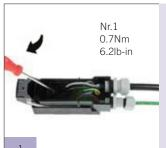
Open the cover. Put the cable gland on the round cable. Cut the round cable to the desired length and remove the sheath. Introduce the leads after having stripped off the insulation and tighten the clamping screws. Check if the O-ring seal is at the right position and tighten the cable gland.
