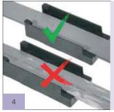
Position the asymmetric fl at cable (right position is shown by the groove in one narrow side of the cable sheath). Is the fl at cable not in the right position, it cannot be inserted into the base. The cable has to be clean, undamaged, free from grease and oil residue.
