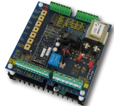
Model 1600i, up to 3HP 6.1" x 6.1" x 3.4" (150 x 150 x 85 mm)
