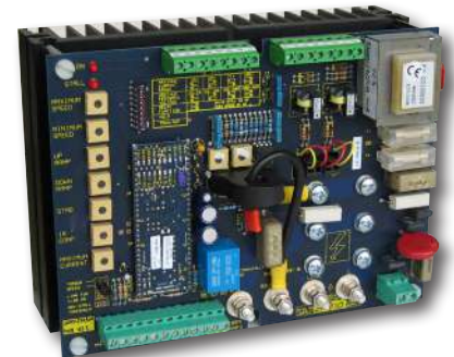
Model 3200i, up to 7.5HP 6.1" x 8.0" x 4.2" (150 x 200 x 105 mm)
